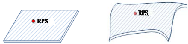
(a) Plane RPS point (b) Surface RPS point Fig.2. The diagrammatic sketch of surface of the RPS points
