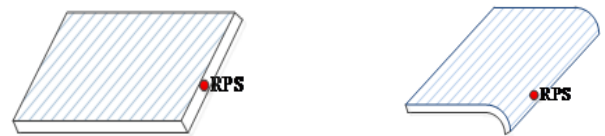
(a) Trimming RPS point (b) Flanging RPS point Fig.3. profile (contour edge) RPS points
